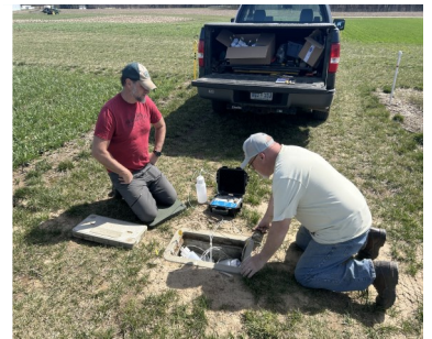
David Weed (left) and Kevin Kahmark (right) installing lysimeters in the ACSE.
